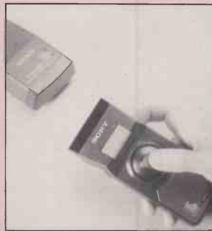
An infrared sensor attaches to the computer so that you can use the joystick from across the room.
